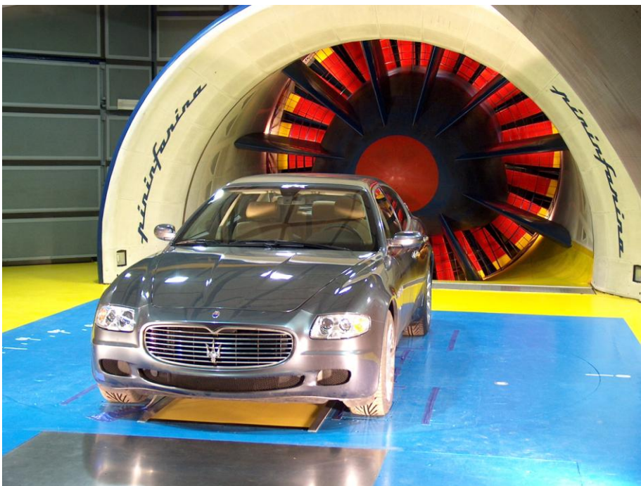
View (in flow direction) into the collector and onto the fan; the moving belt between the wheels (orange) is visible.
